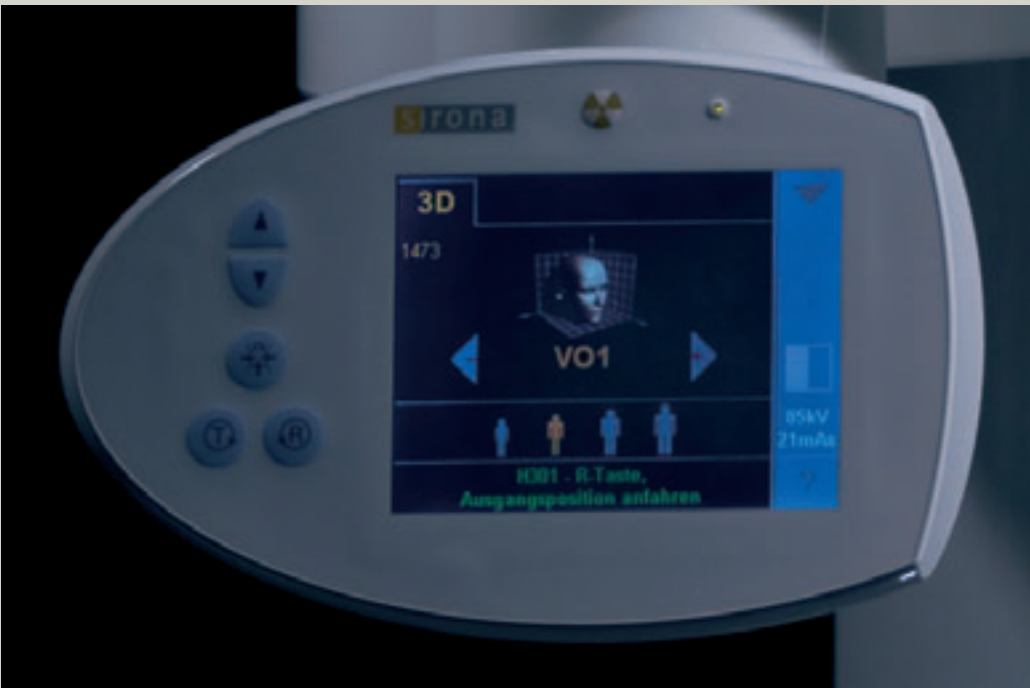
Ease of operation is improved with the GALILEOS Easypad touchscreen 3D: Intuitive control and operator assistance is driven by icons and interactive messages.
